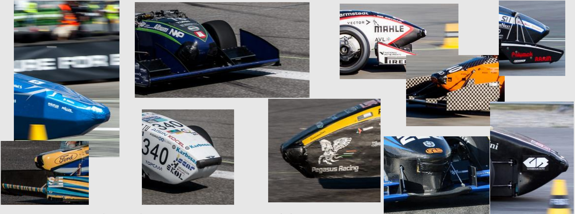
Picture 5: Examples of wrong front body work radii seen at FS Germany 2016
