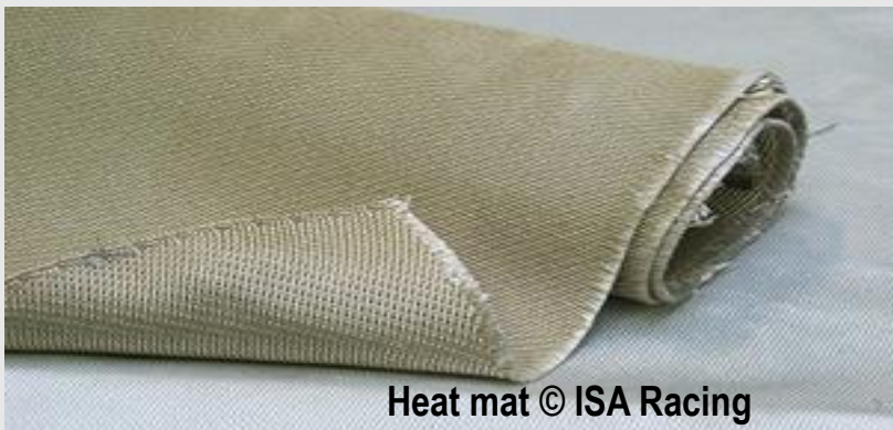
Picture 7: Examples of right and accepted fire wall materials
