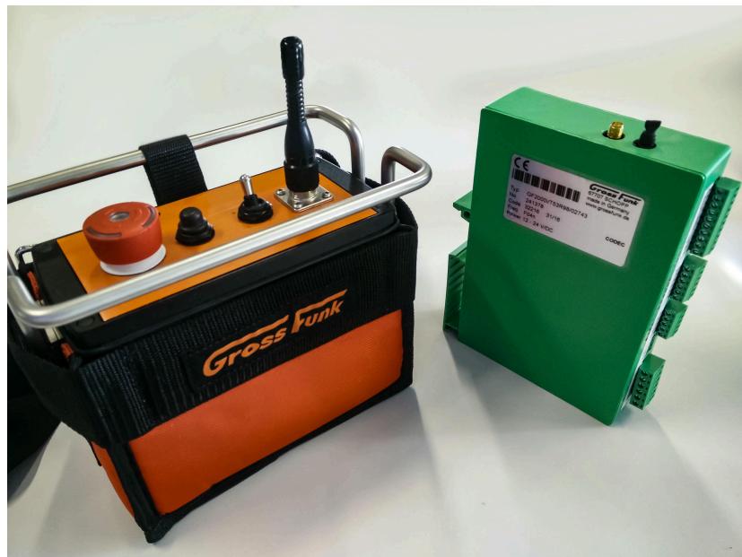
Figure 6: RES sender & receiver
