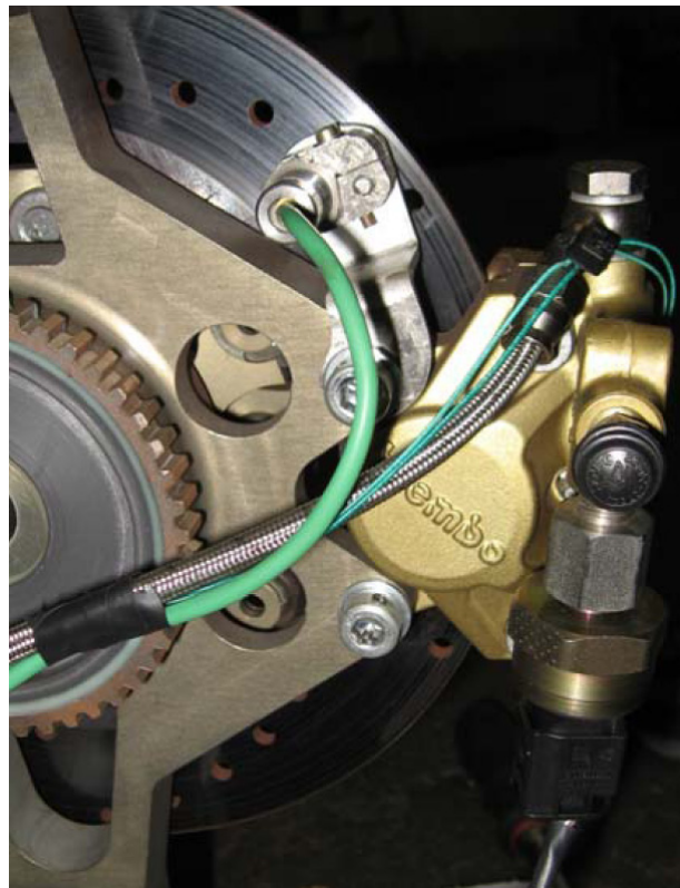
Figure 30: Mounting of the brake disc's temperature sensor at the BRC08 [6]
