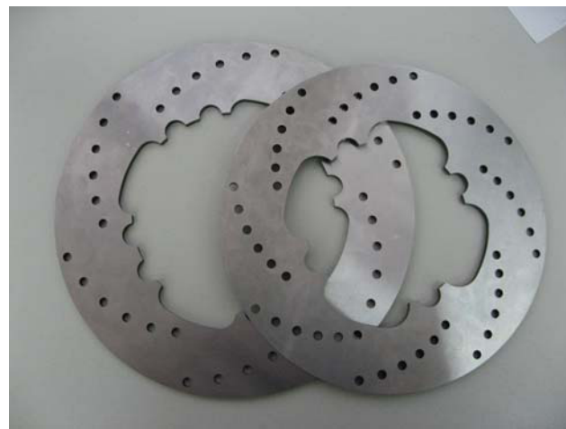
Figure 25: Friction ring grinded BRC08 [6]
