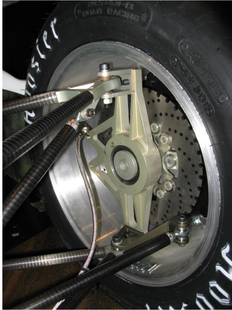
Figure 27: Alternative brake disc – front axle BRC09
