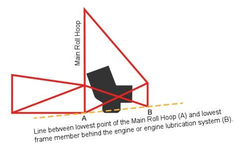
The engine lubrication system must be protected from surface contact in any situation while in operation on track, especially in the event of a suspension failure. The skid plate itself can not be mounted to parts of the engine.
