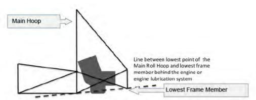
The engine lubrication system must be protected from surface contact in any situation while in operation on track, especially in the event of a suspension failure. The skid plate itself can not be mounted to parts of the engine
