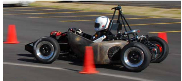
Clad with a see-through fiberglass body, F15 rounds a skidpad course for suspension testing prior to competition in Detroit.
